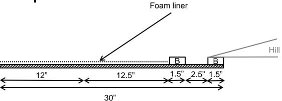
One 30" x 12", 1/4" plywood piece Two 12" x 1.5" x 0.75" wood blocks 0.75" screws to connect wood together Duct tape to connect hill to landing (shown on left) and around edges of plywood
