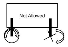
No wheels, treads or any item that touches the ground may rotate around its axle as it's primary source of motion. Axle rotation to move legs is perfectly acceptable.
