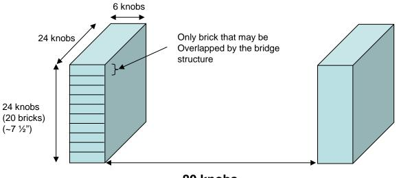
Note: The support structures may be built Differently than shown here. However, any Alterations may not affect the inside span, The top surface, or the top two bricks of the Support.
