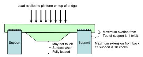
The central portion of the bridge may extend beyond the One brick support restriction, however at all points around The support, the overlap may not exceed 1 brick.
